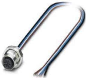
Sensor/actuator flush-type plug, 4-pos., stainless steel design, rear/screw mounting with Pg9 thread, with 0.5 m TPE litz wire, 4 x 0.34 mm 2
