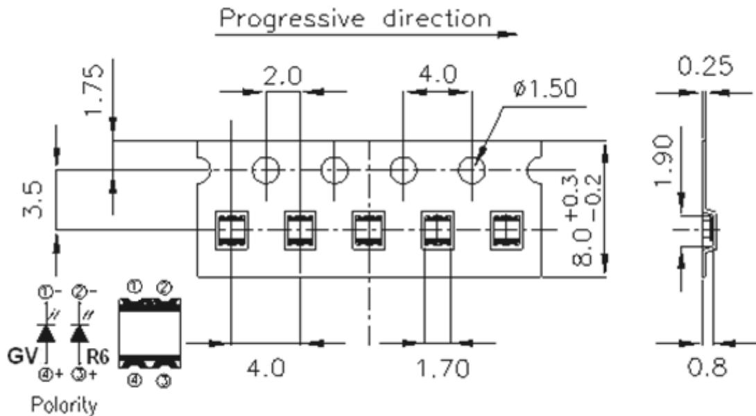
Note: The tolerances unless mentioned is  $\pm 0.1\text{mm}$ , Unit = mm
