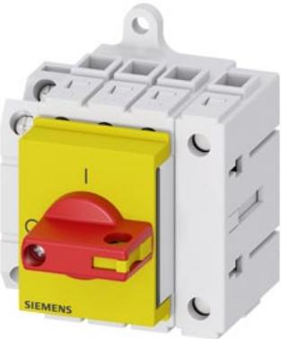
Load disconnector 3LD3, Iu 32 A Main switch 3-pole + N Rated operating capacity for AC-23 A at 400V 11.5kW Installation in distribution boards, Basic switch with selector knob red / yellow with auxiliary switch 1OE + 1S
