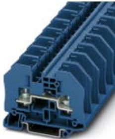
Feed-through terminal block with bolt connection, cross section: 0.1 - 6 mm<sup>2</sup>, AWG: 26 - 10, width 16.3 mm, color: Gray
