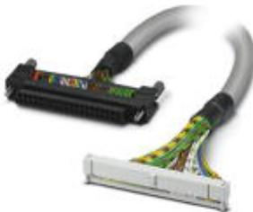
Round cable set; Controller: Siemens S7-300 (6ES7 322-1BP00-0AA0 and 6ES7 322-1BP50-0AA0 (negative switching)); Connection 1: Fujitsu connector (1x 40-position); Connection 2: IDC/FLK socket strip (1x 50-position); Cable length: 1 m
