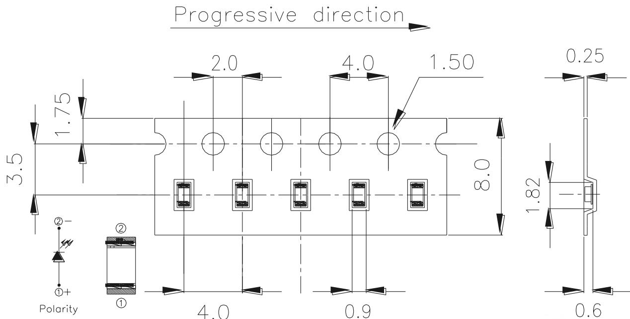
Note: The tolerances unless mentioned is  $\pm 0.05\text{mm}$ , Unit = mm
