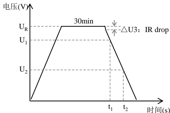
$$\text{容量计算公式: } C = \frac{I \times (t_2 - t_1)}{U_1 - U_2}$$
