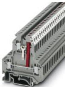
Component terminal block, Connection type: Screw connection, Cross section: 0.2 mm<sup>2</sup> - 4 mm<sup>2</sup>, AWG: 24 - 12, Nominal current: 32 A, Nominal voltage: 500 V, Length: 56 mm, Width: 6.2 mm, Color: gray, Assembly: NS 35/7,5, NS 35/15, NS 32
