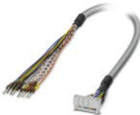
Round cable set; connection 1: Single wires (14-position) (The wires are marked and fitted with ferrules.); connection 2: IDC/FLK socket strip (1x 14-position); cable length: 0.5 m
