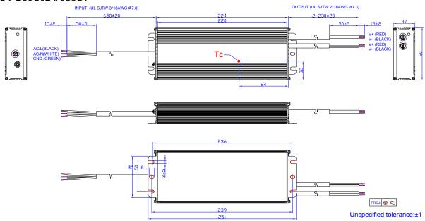
**Note:** The 2 DC output cables are connected in parallel internally because one AWG #18 wire can only carry 10A. Please connect the 2 red wires together and 2 black wires together in application, or ensure each cable carries same current.
