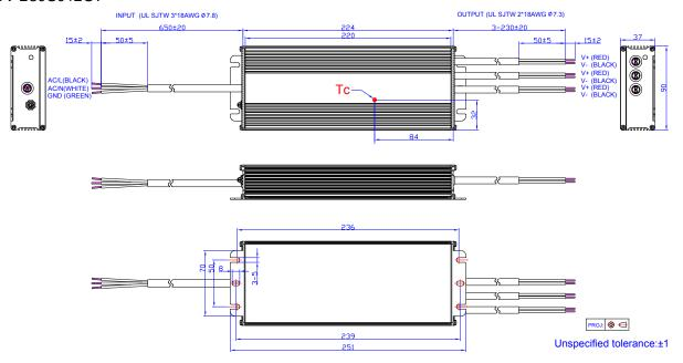
**Note:** The 3 DC output cables are connected in parallel internally because one AWG #18 wire can only carry 10A. Please connect the 3 red wires together and 3 black wires together in application, or ensure each cable carries same current.
