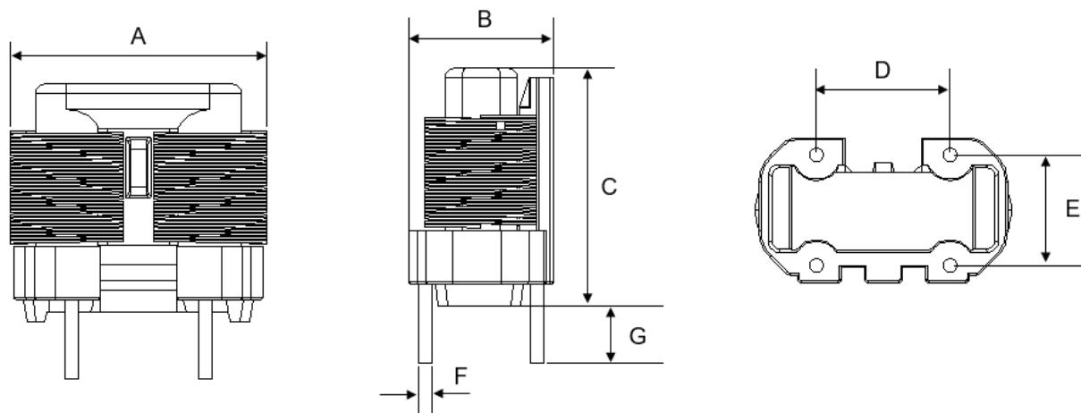
PCB aperture  $\geq \Phi 1.2\text{mm}$
