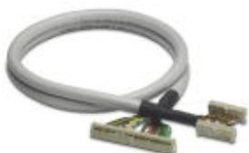
Round cable set; controller: Emerson Delta V; connection 1: IDC/FLK socket strip (2x 20-position); connection 2: IDC/FLK socket strip (1x 50-position); cable length: 10 m
