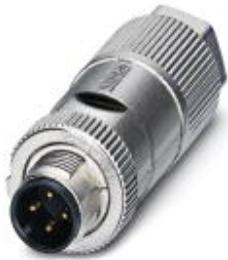
Bus system connector, PROFIBUS PA (31.25 kbps), 2-position, halogen-free, shielded, Plug straight M12 SPEEDCON, Insulation displacement connection, knurl material: Zinc die-cast, nickel-plated, external cable diameter 5 mm ... 9.7 mm
