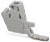
Pick-off terminal block, nom. voltage: 1000 V, nominal current: 32 A, connection method: Screw connection, number of connections: 1, cross section: 0.14 mm<sup>2</sup> - 6 mm<sup>2</sup>, AWG: 26 - 10, width: 8.1 mm, height: 24.7 mm, color: gray, mounting type: on base element
