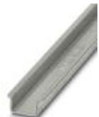
DIN rail, unperforated, Standard profile 2.3 mm, width: 35 mm, height: 15 mm, acc. to EN 60715, material: Steel, galvanized, passivated with a thick layer, length: 2000 mm, color: silver
