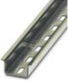
DIN rail perforated, Standard profile, width: 35 mm, height: 15 mm, similar to EN 60715, material: Steel, galvanized, passivated with a thick layer, length: 2000 mm, color: silver
