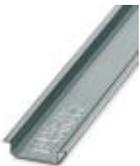
DIN rail, unperforated, Standard profile, width: 35 mm, height: 7.5 mm, acc. to EN 60715, material: Steel, Galvanized, white passivated, length: 2000 mm, color: white
