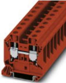
Feed-through terminal block, nom. voltage: 1000 V, nominal current: 76 A, connection method: Screw connection, number of connections: 2, cross section: 1.5 mm<sup>2</sup> - 25 mm<sup>2</sup>, AWG: 16 - 4, width: 12.2 mm, height: 54.4 mm, color: red, mounting type: NS 35/7,5, NS 35/15
