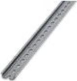
DIN rail perforated, Standard profile, width: 35 mm, height: 7.5 mm, acc. to EN 60715, material: Steel, Galvanized, white passivated, length: 2000 mm, color: white
