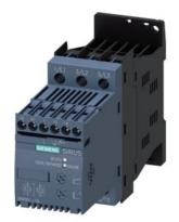
SIRIUS soft starter S00 17.6 A, 7.5 kW/400 V, 40 °C 200-480 V AC, 110-230 V AC/DC Screw terminals
