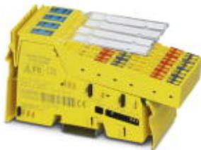
Safety-related digital input module, IP20 protection, for the SafetyBridge V3 and PROFIsafe system. The module has 8 safe digital inputs for two-channel assignment or 16 safe digital inputs for single-channel assignment.
