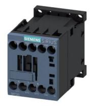
power contactor, AC-3e/AC-3, 12 A, 5.5 kW / 400 V, 3-pole, 230 V AC, 50/60 Hz, auxiliary contacts: 1 NC, screw terminal, size: S00  $\,$
