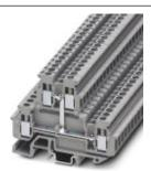
Mini feed-through terminal block, With equipotential bonder, Cross section: 0.2 mm<sup>2</sup> - 4 mm<sup>2</sup>, AWG: 24 - 12, Connection type: Screw connection, Width: 5.2 mm, Color: gray, Mounting type: NS 15, NS 35/7,5, NS 35/15
