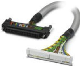
Round cable set; controller: MODICON® M340 (BMX DDI 3202K, BMX DDI 6402K, BMX DD0 3202K, BMX DD0 6402K, BMX DDM 3202K); connection 1: Fujitsu connector (1x 40-position); connection 2: IDC/FLK socket strip (1x 50-position); cable length: 3 m
