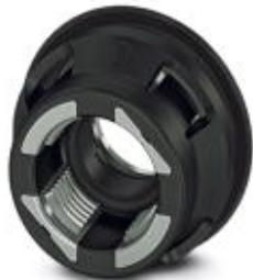
M12 housing screw connection with tolerance-compensating function, for straight THR solderable M12 socket contact inserts. Suitable for 1.0 mm ... 1.8 mm thick front plates.
