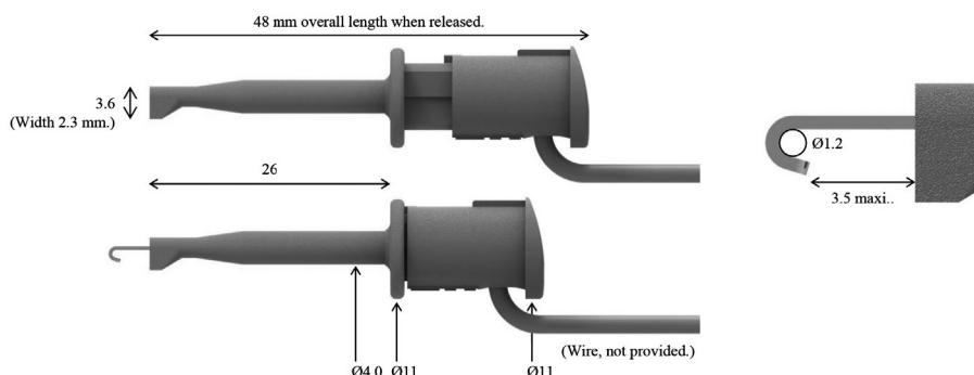
The hook fits to 1.2mm diameter round pins and 0.9mm x 0.9mm square pins. The gold plating prevents oxidation and keeps good electrical conductance.
