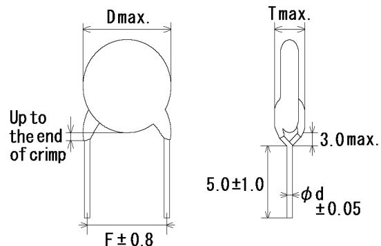
Note) The mark '\*' of lead code differ from lead spacing(F) and lead diameter(d).
