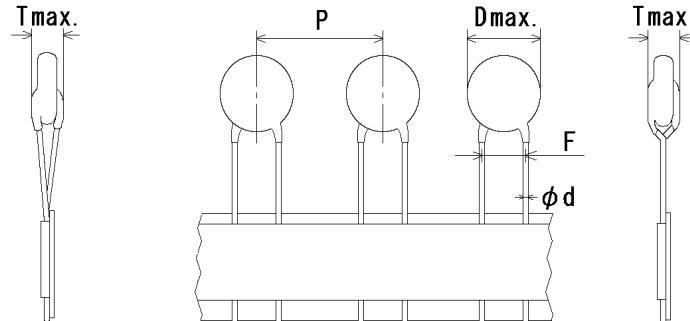
Note) The mark '\*' of lead code differ from lead spacing(F), lead diameter(d) and pitch of component(P).
