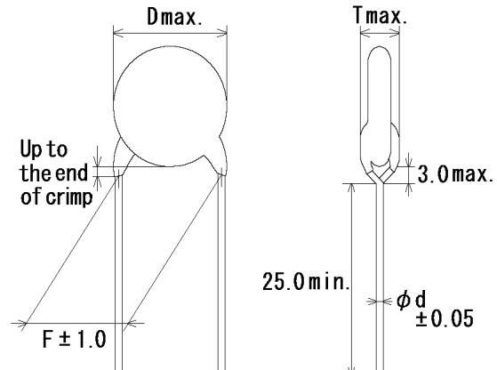
Note) The mark '\*' of lead code differ from lead spacing(F) and lead diameter(d).
