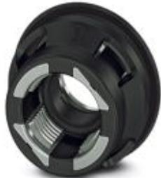
M12 housing screw connection with tolerance-compensating function, for straight, THR solderable M12 socket contact inserts. Suitable for 1.7 mm ... 2.5 mm thick front plates.
