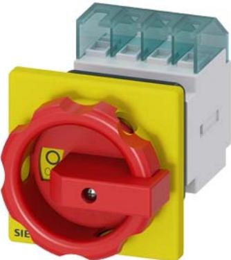
SENTRON, Switch disconnector 3LD, emergency switching-off switch, 4- pole, Iu: 16 A, operating power / at AC-23 A 400 V: 7.5 kW, front-mounted, rotary operating mechanism, Red / yellow, central mounting 22.5 mm of the handle
