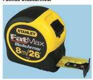
Extra wide 1¼ inch blade for easier reading and 11 feet of stand-out, constructed with a 3m industrial thermoplastic coating for maximum durability and reduced breakage. Impact blade is mylar coated for long life and features a 3 rivet corrosion resistant end hook, which gives true zero reading and accurate inside and outside measurement. The end hook is also multifunctional allowing grip on side, top and bottom.
