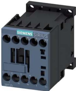
power contactor, AC-3, 9 A, 4 kW / 400 V, 4-pole, 24 V DC, main contacts: 2 NO + 2 NC, screw terminal, size: S00
