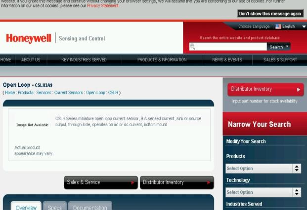
Honeywell □s CSLH Series miniature, open-loop current sensors incorporate our SS490 Series miniature ratiometric linear Hall-effect sensor (MRLD). The sensing element is encapsulated in a printed circuit boardmountable plastic package. The combination of sensor, flux collector and housing comprises the current sensor assembly. These sensors are ratiometric.
