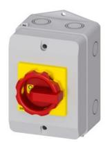
SENTRON, Switch disconnector 3LD, emergency switching-off switch, 3- pole, lu: 16 A, operating power / at AC-23 A 400 V: 7.5 kW, Molded plastic encapsulation for metric cable gland, 1 NC, 1 NO, rotary operating mechanism, red/yellow
