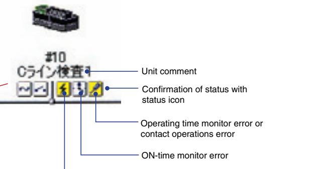
The diagram shows a slave unit with a unit comment "Cライン検査" and several status icons. A legend on the right explains the symbols: a blue box for unit comment, a green box with a checkmark for confirmation of status with status icon, a red box for operating time monitor error or contact operations error, a yellow box for ON-time monitor error, and a blue box for ON-time power supply voltage monitor error.
