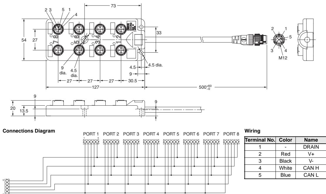
● Environment-resistive Models for Thick Wires with 7/8-16UN Mini Connectors
