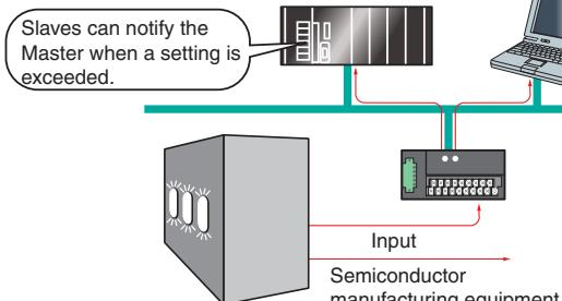
The peaks or valleys of temperature inputs that change in a regular pattern are counted to predict when devices operating with severe temperature swings are due for maintenance.
