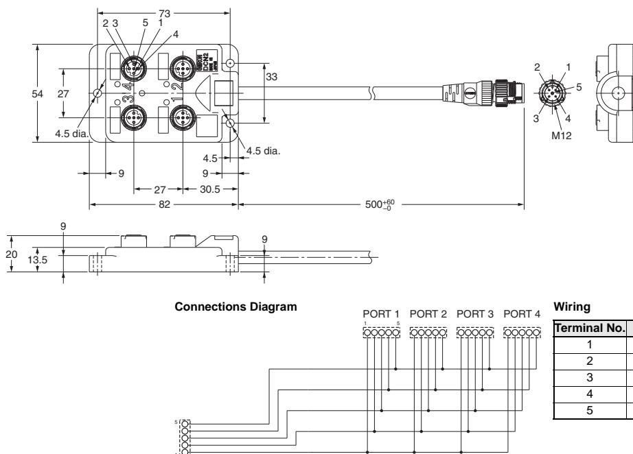
**Shielded Branch Relay Box with Eight Ports**
