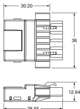
**Conversion Connector for Standard Thin Cable and Flat Cable**
