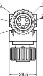
**T-branch Connector (5 Conductors for Communications,
