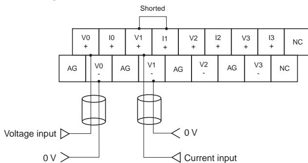
**Note:** With using a current input, always short the V+ and I+ terminals.
