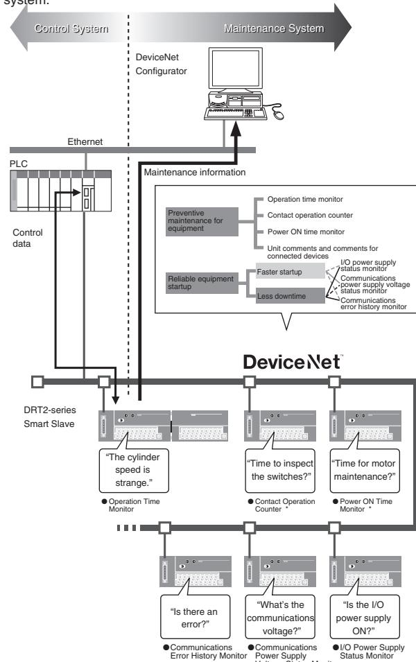
\*You cannot use the contact operation counter and the power ON time monitor at the same time.
