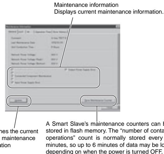
Depending on the maintenance information that has been generated, more details can be viewed by clicking the **OUT** tab, **IN** tab, or **Operation Time** tab.
