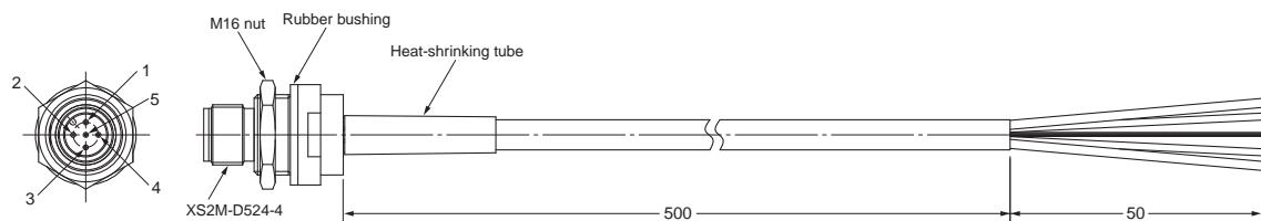
**Panel-mounting Connector (Socket), Solder-cup Terminals**
