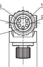
**Connector (Plug) with Terminating Resistance**
