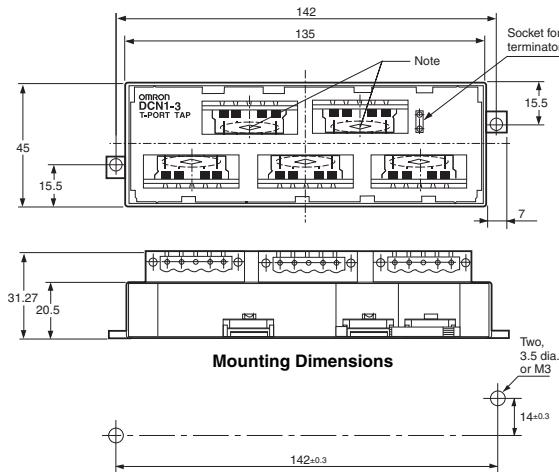
**Note:** When connecting a branch line to the main line, connect the main line to the connector marked with an asterisk because the resistance between the asterisked portion is minimal.
