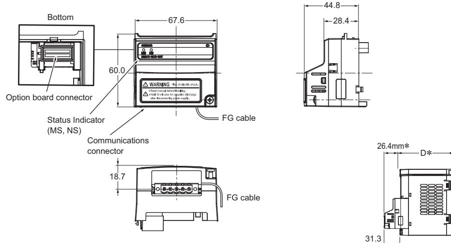
\* After the DeviceNet Communication Unit is installed, dimension D of the inverter increases by 26.4 mm.
