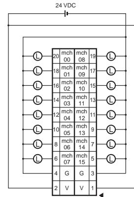
Wiring Diagram of Connector Cable Provided with the DRT2-ID16ML(-1) and DRT2-OD16MLX(-1)
