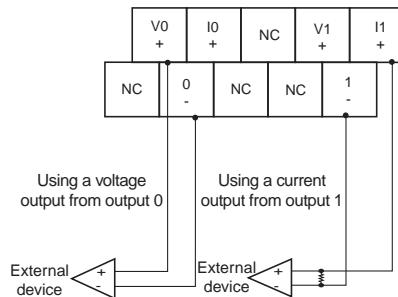
**Note:** The voltage and current output ranges (signals) are set with either the DIP switch or the Configurator settings.
