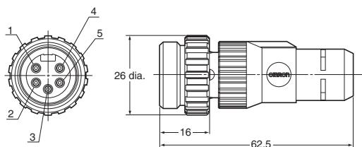
**Panel-mounting Connector (5 Pins for Communications)**
