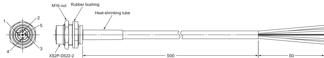
**Panel-mounting Connector (Socket), Solder-cup Terminals**
