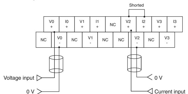
**Note:** With using a current input, always short the V+ and I+ terminals.
