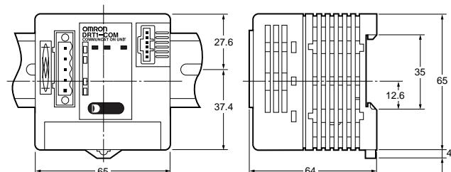
Note: The Unit is shown with the end connector mounted in the above diagram.
