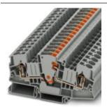
Test disconnect terminal block, connection method: Spring-cage connection, cross section: 0.2 mm² - 10 mm², AWG: 24 - 10, width: 8.2 mm, color: gray
