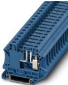
Disconnect terminal block, With test socket screws for insertion of test plugs, Connection type: Screw connection, Cross section: 0.2 mm<sup>2</sup> - 10 mm<sup>2</sup>, AWG: 24 - 8, Nominal current: 20 A, Nominal voltage: 500 V, Length: 57.8 mm, Width: 8.2 mm, Color: blue, Assembly: NS 35/7,5, NS 35/15
