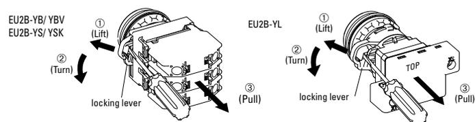
When the contact unit is removed from the emergency stop switch operator, the NO contact closes and the NC contact opens.
