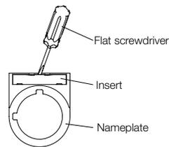
To remove the Insert, insert a flat screwdriver between the Insert and Nameplate.
