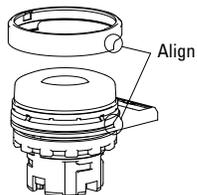
To remove the rubber boot from the flush and extended pushbuttons, gently insert the slotted screwdriver (0.5t x 4w or below) inside a notch on the rubber boot holder and tilt to the direction shown by the arrow ①. To prevent damage, do not apply excessive force to the EU2B when removing the rubber boot.
