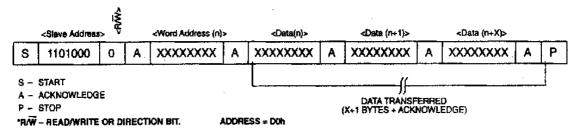
2. **Mode of «slave» receiver (write mode from HT1307):** The first byte is received and processed as in the mode of the «slave» receiver. However, in this mode the direction bit will signify, that the transmission direction is changed. HT1307 sends the serial data by SDA, the cycle pulses - by SCL. statuses START and STOP are understood as the beginning and end of the consecutive transmission. The address byte is the first byte, received after occurrence of the status START,
