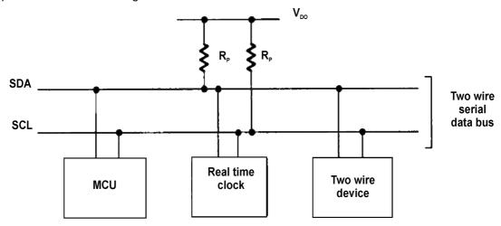
Data transfer can be initiated only when the bus is not occupied. In the process of the data transfer the data line should remain stable, while the line of the cycle signal is in the high status. Status alterations of the data line at that moment, when the cycle line is in the high status, will be regarded as the control signals.
