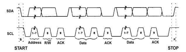
Depending on the status of bit  $R/\overline{W}$ , there are possible two types of transfer:
