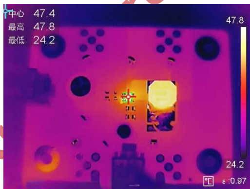
图 13 热性能 ( V_{IN} = 12V , V_{OUT} = 5V , I_{OUT} = 1A )
