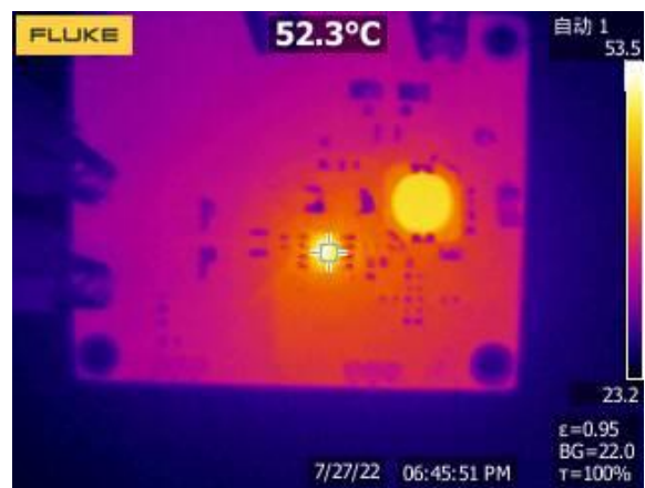
Figure 24. Thermal, 48VIN, 12Vout, 1.2A
