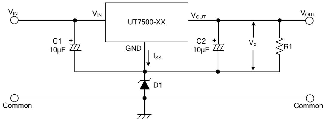
$$V_{OUT} = V_X + V_{D1}$$
