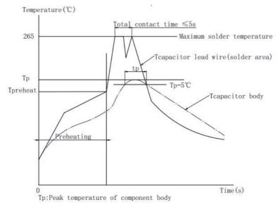
A Because overheating could damage the capacitor, we recommend paying attention to the maximum capacitor temperature and heating time, use temperature sensor to detect the maximum capacitor body temperature.
