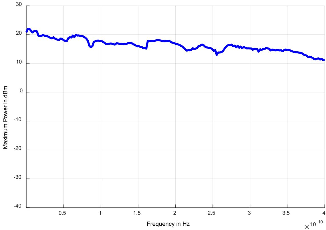
**Max Output Power 0.01 to 40 GHz (with option PE2)**
