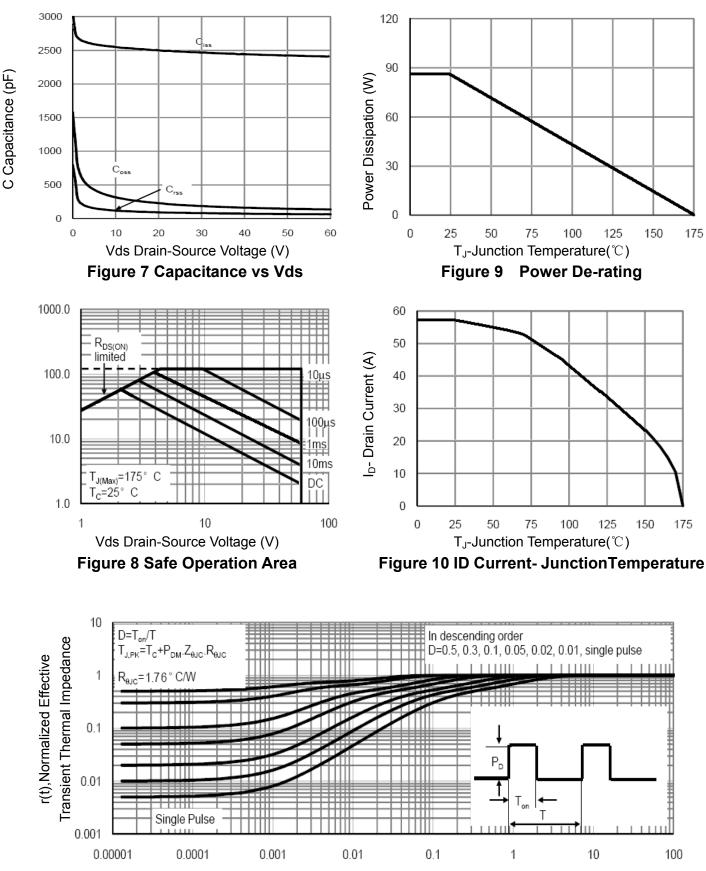
Square Wave Pluse Duration(sec) Figure 11 Normalized Maximum Transient Thermal Impedance
