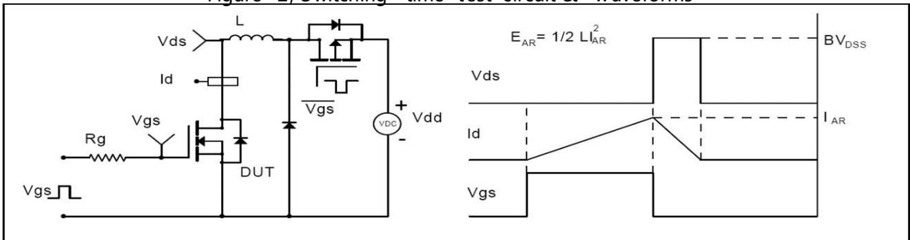
Figure 3, Unclamped inductive switching (UIS) test circuit & waveforms
