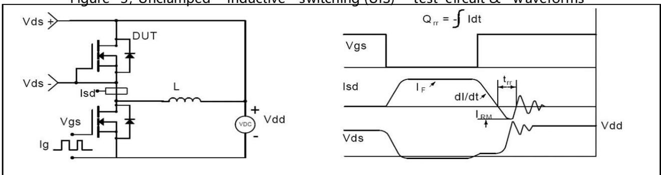
Figure 4, Diode reverse recovery test circuit & waveforms
