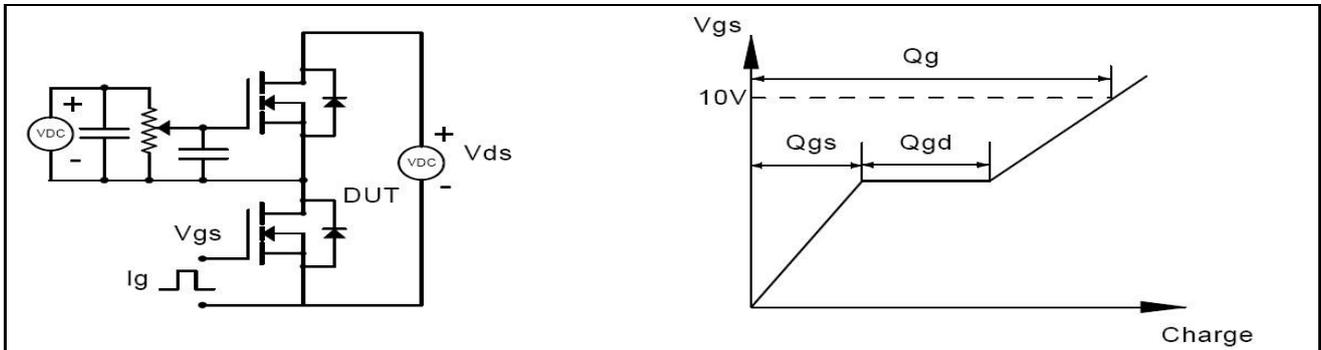
Figure 1, Gate charge test circuit & waveform
