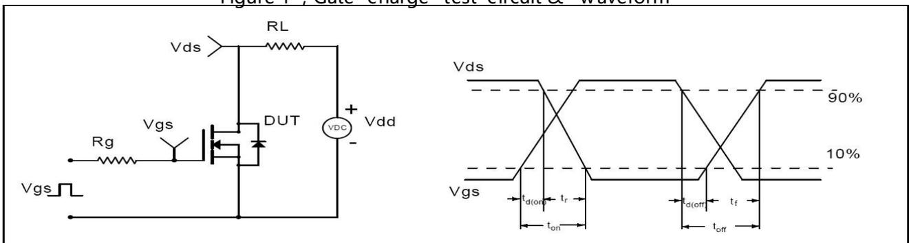
Figure 2, Switching time test circuit & waveforms
