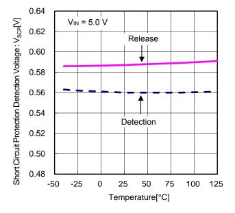
Figure 17. Short Circuit Protection Detection Voltage
