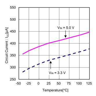
Figure 4. Circuit Current vs Temperature
