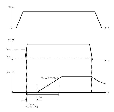
Figure 19. Enable ON/OFF Timing Chart
