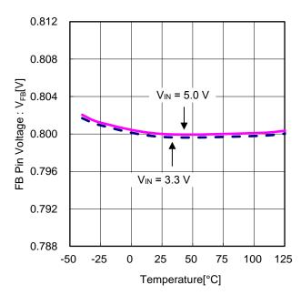
Figure 6. FB Pin Voltage vs Temperature
