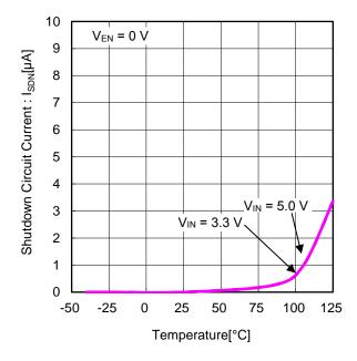
Figure 3. Shutdown Circuit Current vs Temperature
