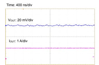
Figure 53. Load Transient Response  $(I_{OUT} = 0 A \leftrightarrow 1 A)$
