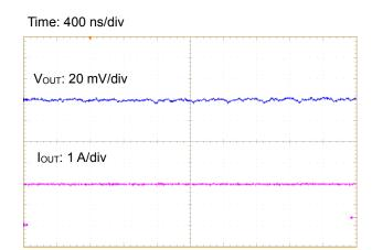
Figure 38. Load Transient Response  $(I_{OUT} = 0 A \leftrightarrow 1 A)$
