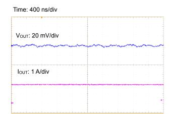
Figure 43. Load Transient Response ( $I_{OUT} = 0 A \leftrightarrow 1 A$ )
