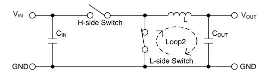
Figure 56. Current Path when H-side Switch = OFF, L-side Switch = ON
