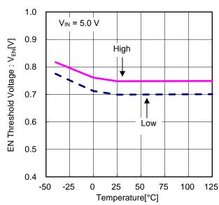
Figure 13. UVLO Detection Voltage vs Temperature
