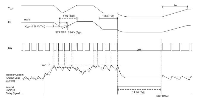
Figure 22. Short Circuit Protection (SCP) Timing Chart
