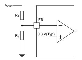
Figure 26. Feedback Resistor Circuit
