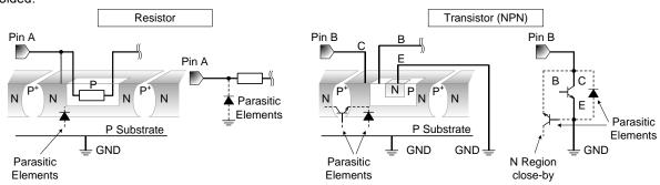
Figure 60. Example of Monolithic IC Structure
