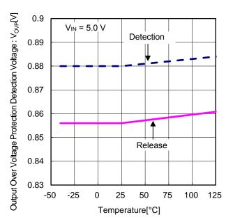
Figure 18. Output Over Voltage Protection Detection Voltage vs Temperature
