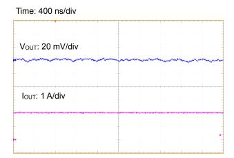
Figure 33. Load Transient Response ( $I_{OUT} = 0 A \leftrightarrow 1 A$ )
