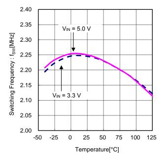
Figure 5. Switching Frequency vs Temperature
