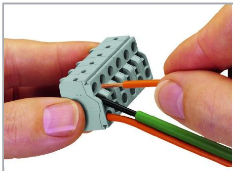
Operating Push-in CAGE CLAMP® is easy, fast and identical to that of CAGE CLAMP®. The screwdriver is fully inserted into the operating slot, holding Push-in CAGE CLAMP® open. After the conductor has been inserted into the clamping unit and the screwdriver been withdrawn, the conductor is clamped safely. Solid and fine-stranded conductors  $< 0.5 \text{ mm}^2$  (20 AWG) are terminated and removed using a screwdriver.
