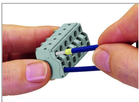
Solid conductors  $\geq 0.5 \text{ mm}^2$  (20 AWG), as well as ferruled, fine-stranded conductors can be terminated by simply pushing them into unit. Integrated test ports allow touch contact with current bar via test probes in both horizontal and vertical directions.
