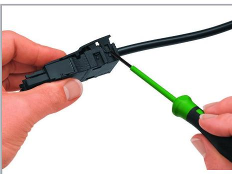
Push down strain relief clamp via screwdriver (2.5 mm blade width) alternately on both sides.
