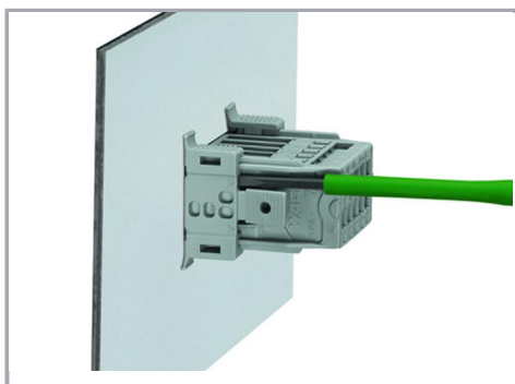
For removal, insert operating tool (2.5 mm blade) into release slot.
