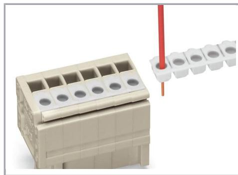
Conductors with small cross-sections are highly flexible, and they deform when pushed against the conductor stop in connectors. As a result, the conductor insulation – not the copper conductor – may be clamped, causing intermittent contact or no contact at all. The solution: an insulation stop for CAGE CLAMP®-equipped 734 Series Male and Female Connectors.
