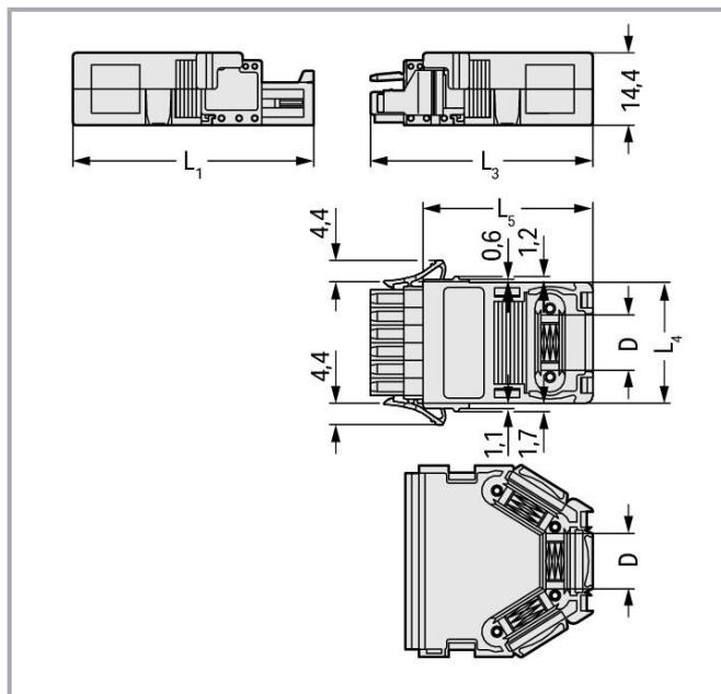
Strain Relief Housing Dimensions (in mm):
