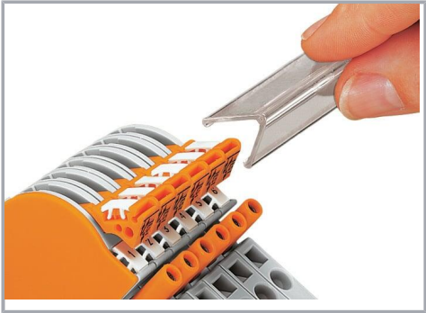
Snapping transparent locking cover onto 1–8 disconnect links: a) Mechanically lock several links for multi-pole switching applications b) Protect markers
