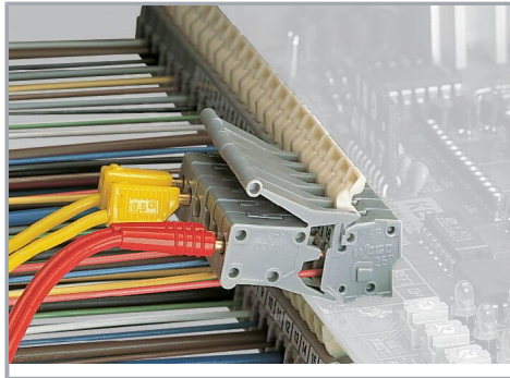
Testing with test plug modules.
