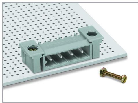
Locking devices enhance connection reliability between male headers with angled solder pins and the PCB. This substantially reduces mechanical stress on both solder pins and joints, particularly when dealing with small lengths and frequent mating cycles.
