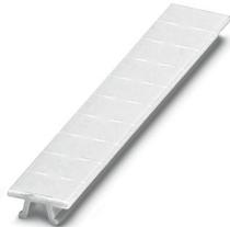
Zack marker strip, Strip, white, unlabeled, can be labeled with: PLOTMARK, CMS-P1-PLOTTER, mounting type: snapped, for terminal block width: 6.2 mm, lettering field size: 6.15 x 10.5 mm, Number of individual labels: 1000
